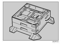
Adjust the four corners of the printer to those of the 1000sheet paper feed unit, and then slowly lower the printer into place.
